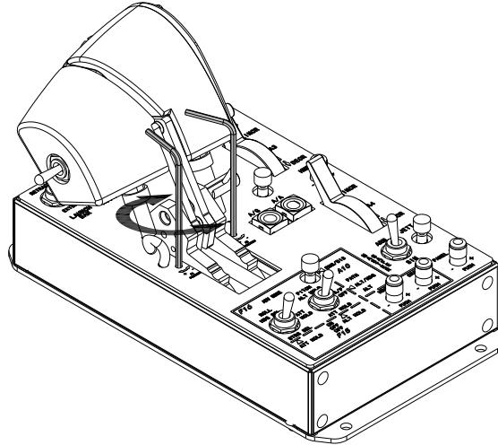
Use the allen wrench to adjust friction. Clockwise for increase friction, CCW for decrease friction
