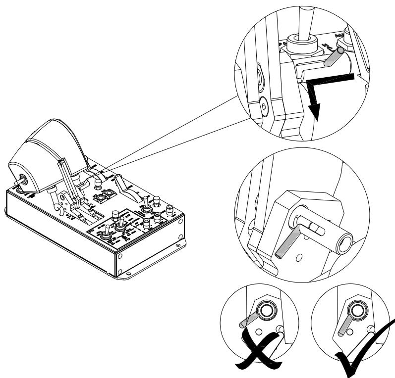
Align the grip and engage the sync lock to the position shown in picture for connected operation.
